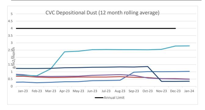
A 12-month rolling average of depositional dust concentrations has been presented below. Dust Gauges DDG001, DDG002, DDG003 and DDG004 are located within a closer proximity to Chain Valley Colliery and DDG006 is positioned in a location representative of the Chain Valley Colliery ventilation fan site at Summerland Point.
